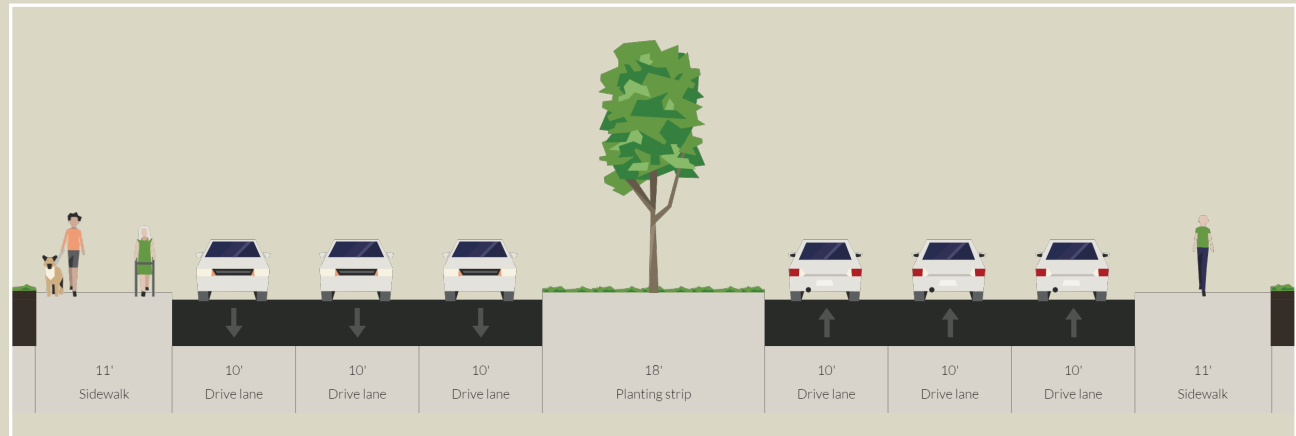
EXISTING SECTION ON POWERLINE ROAD
