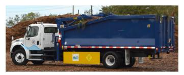
**2017** | Truck Side Guards – Fleet Services installed side guards on 12 new trucks recently purchased for bulk waste collections. The side guards help reduce deaths resulting from "right-hook" crashes by preventing bicyclists from being pulled under the vehicle and also reduce the severity of vehicular crash side collisions.
