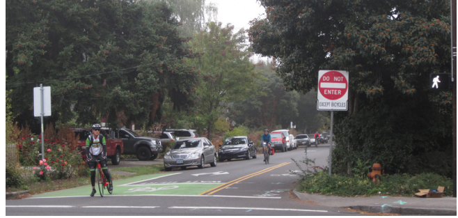
Bicycle box with lead-in bike lane
