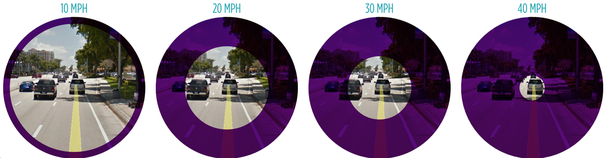
Figure 27 | Driver's Cone of Vision by Travel Speed
