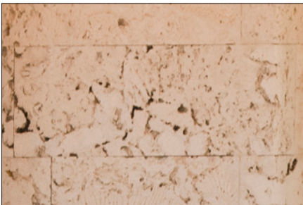
Limestone - A sedimentary rock; typically oolite or keystone in Fort Lauderdale, used for building walls, window sills and lintels, ornamental stone trim, sculpture and for producing lime.
