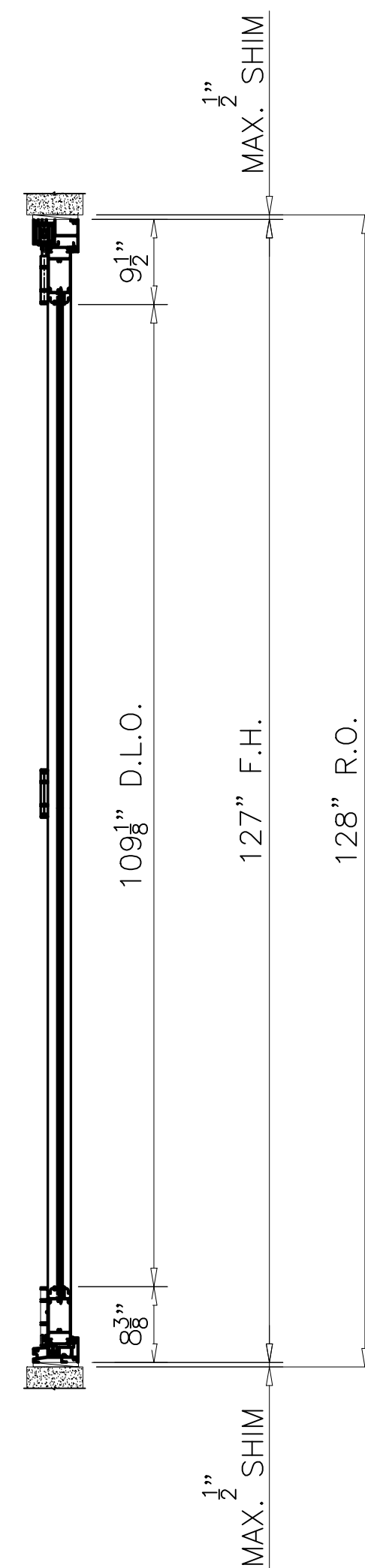
3 SECTION (EXT. HINGES) 200 SCALE 3/4" = 1'-0"
