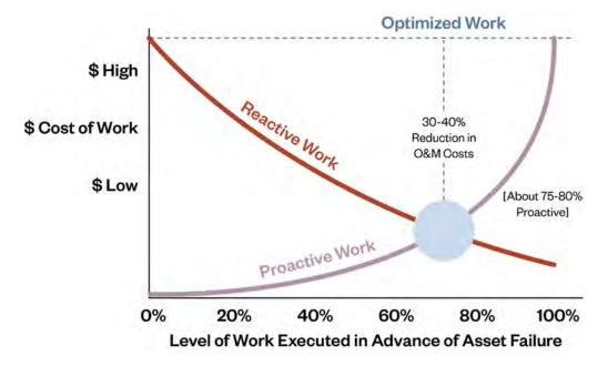
Figure 2.9: Optimized Maintenance: Optimal Mix of Proactive and Reactive Work
