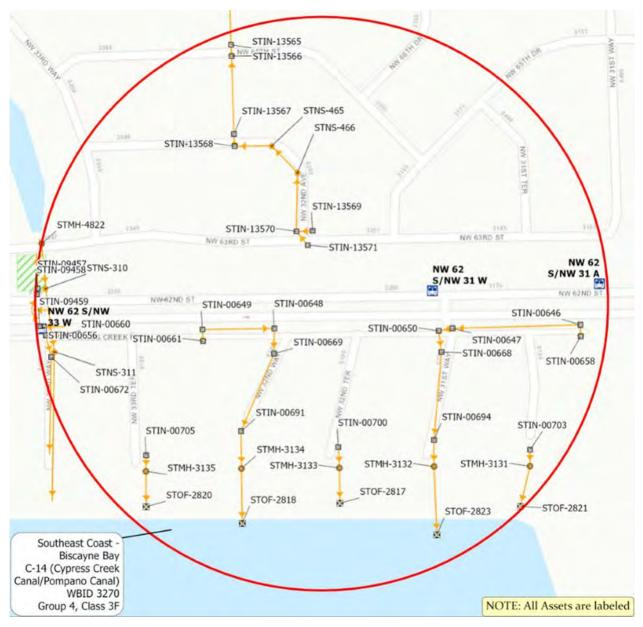
Figure 8.58: Prospect Recharge Watershed Data Subset Used for CoF Analysis
