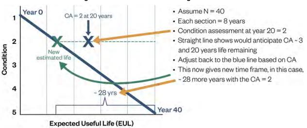
Figure 2.3: Calculation of Remaining Useful Life
