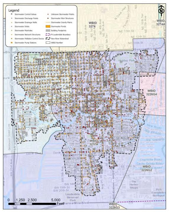
Figure 8.41: Hard Assets in New River Watershed (2019 Stormwater Geodatabase)
