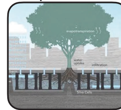
Resiliency - Silva Cells for Stormwater Management
