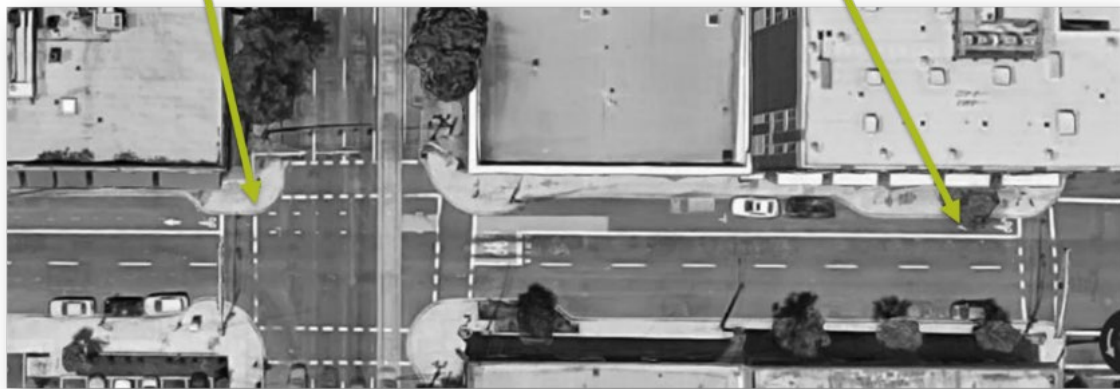
Broadway & N Williams Street, Portland, OR. The bicyclist triggers a detector downstream of the
