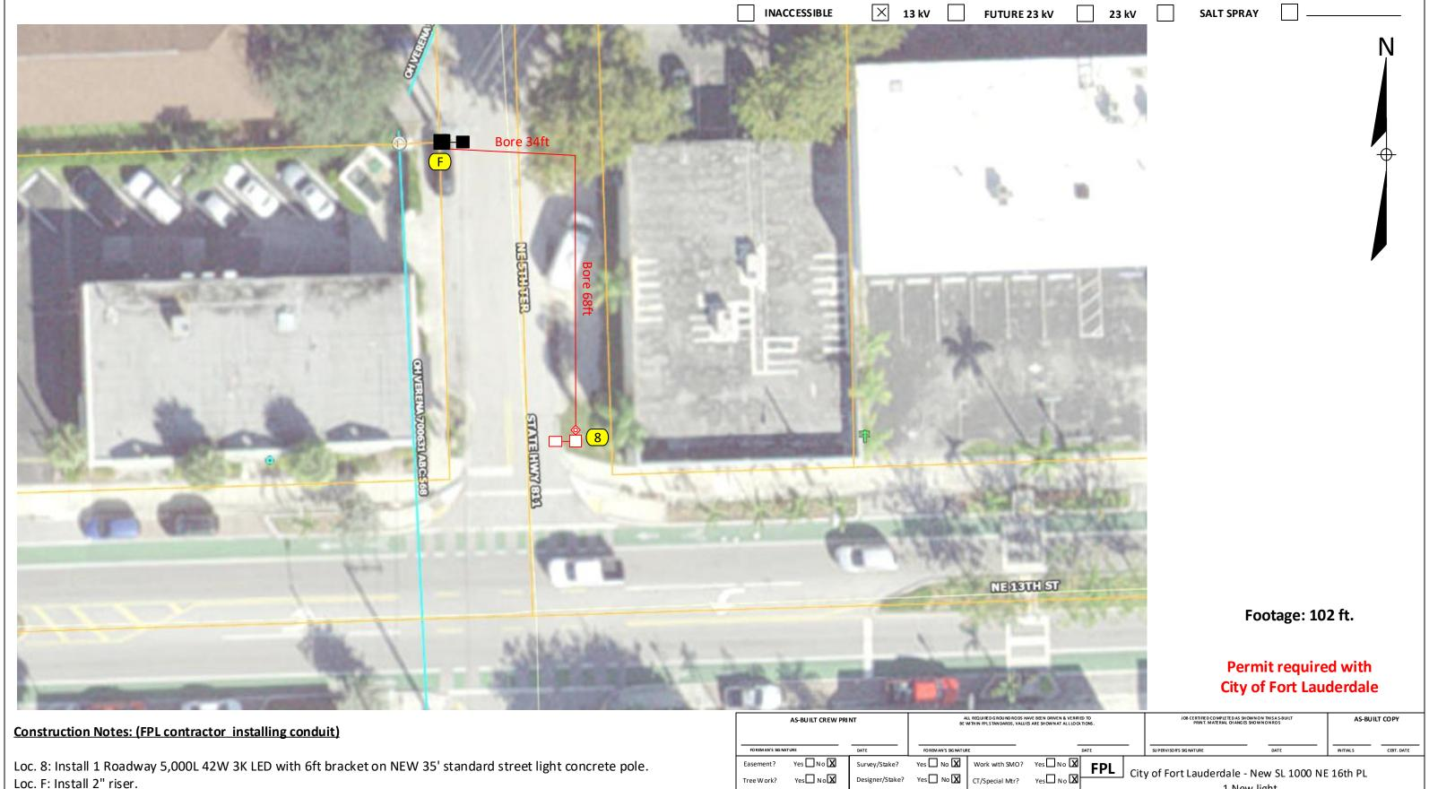
FPL contractor to install 2" flex pipe with 24" minimum cover as shown in the drawing using directional bore. Cable to be used is #6 DPX. FPL contractor installing hand-holes and staking locations of the poles. Pole on this page to be installed in R/W in the back-end of the sidewalk.
