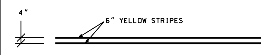
DOUBLE SOLID LINES DETAIL PER FDOT INDEX 711-001 NOT TO SCALE
