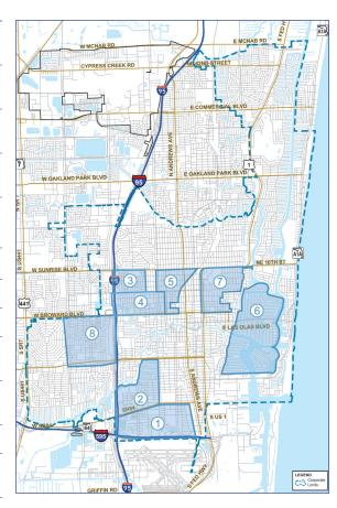
**Stormwater improvements in the Edgewood Neighborhood are almost complete!** New stormwater infrastructure has been added to one of the most vulnerable areas in the City. This infrastructure includes catch basins, gravity piping, exfiltration trenches, swales, outfalls, and tidal valves. The Edgewood system will be fully functional once the River Oaks Pump Stations become operational. The Edgewood project is anticipated to be complete by the end of March, **five months ahead of schedule!**
